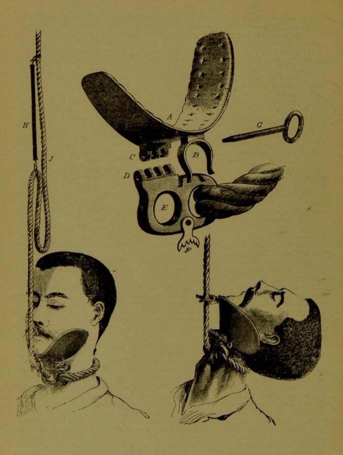
A chin trough; B spring fork for ascending rope; C half hinge; D half hinge; E eyelet for noose; F toothed spring in place of leather washer to prevent noose relaxing: G centre pin to complete hinge; H india-rubber tubing to support trough to thin and keep slack rope in safety; J slack rope representing length of drop (in drawing only about eighteen inches, really three feet).
