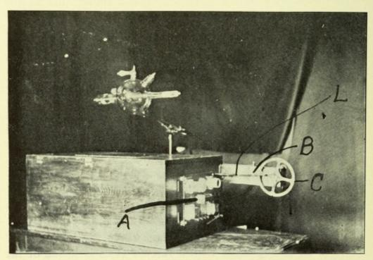
box and cannot be shown on photograph) so that as the handle of the device makes a half turn the pasteboard tube "K" makes a full turn which just winds up 8 inches of film.
