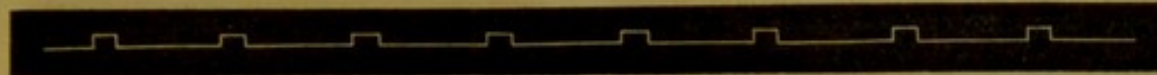
Time tracing. Electro-magnet recording seconds. Applicable to all tracings in Appendix A.
