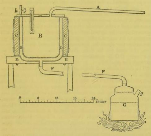
as if broken off), hollowed out to receive it. To this table the vessel is fastened by four small bolts, the extremities of two of which are shown by the sketch. To give a hold to the heads of these bolts, a *flanche* is soldered near the bottom of the outer vessel, which has also a corresponding *flanche* at the top, for the purpose of keeping the packing in its place.
