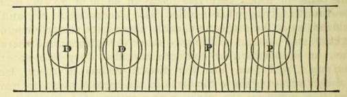
introduced, the lines are opened out as at D. D. In both cases the lines of force are inflected, and a small magnetic needle standing in them at the inflected part would have its direction changed accordingly. Experimental illustrations of these changes in direction are given
