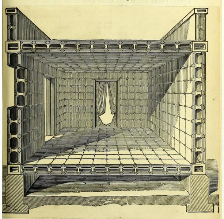
The artist might have curved the upper roof somewhat for the discharge of wet. As against wet, a coating of Val de Travers asphalte, which resists great solar heats, and is uninflammable, would
