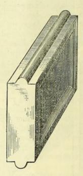
The following is an example of a square pillar support for the lapjointed tiles, where the warmed air is required to be led about:
