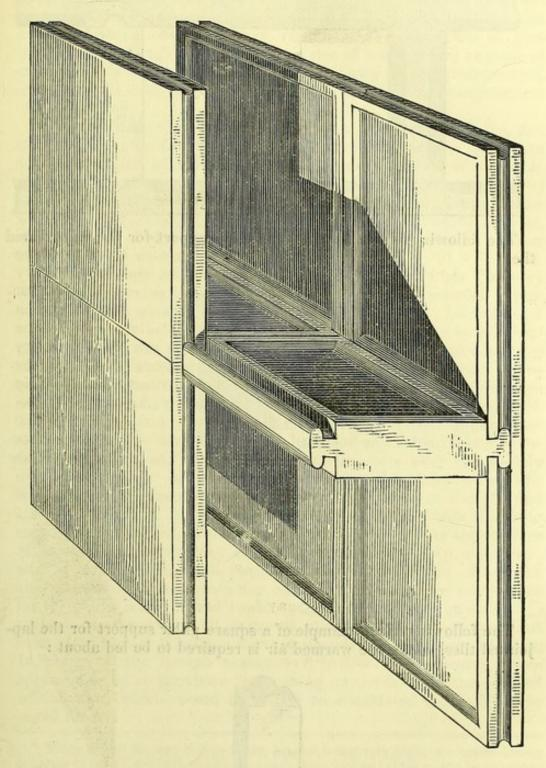
In some cases, in the place of tiles with rabetted joints, tiles with overlap joints may be found eligible, for the application of rapid second mechanical vertical pressure in construction.
