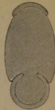
Fig. 7.—Diagrammatic vertical section of forcer and two blades. Shows the dovetailing of forcer with lower blade.
