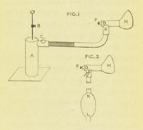
The piston-rod is always raised by means of a helical spring fixed in the upper part of the cylinder, and exhaustion is produced by depressing it with the hand. The capacity
