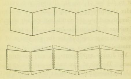
0.00056, so that the relative expansion of the shorter axis is 0.00342 (0.00286 + 0.00056). These changes, which are very curious, may be roughly illustrated by two diagrams, in one of which a series of unexpanded rhombs is arranged longitudinally, and in the other a similar series of rhombs as altered by heat, only with the degree of alteration exaggerated for the sake of distinctness.
