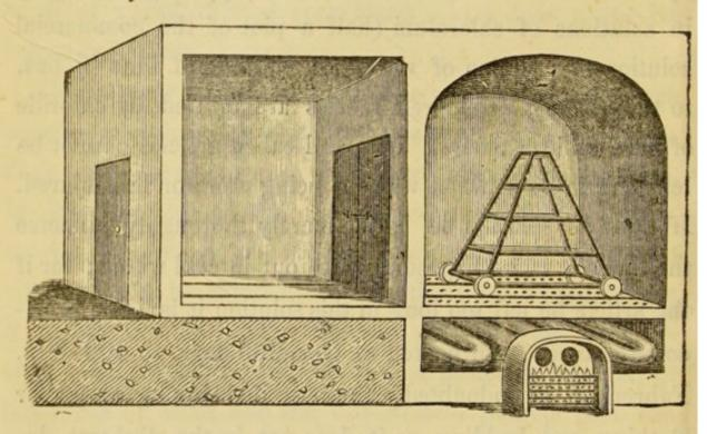
The engraving shows the construction of the chamber. The walls and ceiling of the compartment in which the clothes are heated are built of brick, and its floor is composed of perforated iron plate. The heat is radiated into the compartment from the exterior surface of a coil of iron pipe, 80 feet long, and which acts as part of the furnace
