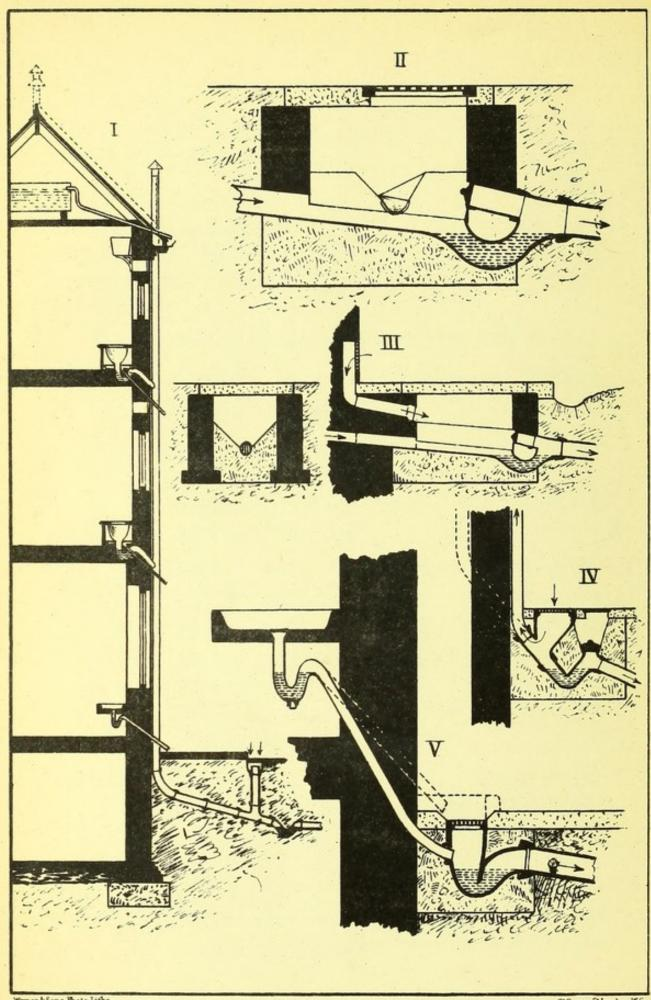
Sewer, so as to prevent the passage of sewer-gas from the Sewer to the house.
