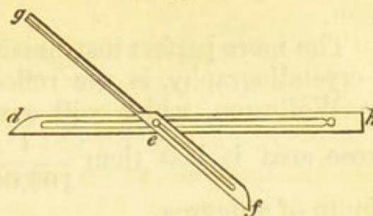
“The common goniometer is a small instrument for measuring this angle,  $g e h$ , of the moveable plates. It consists of a semicircle, fig. 3, divided into 360 equal parts, or half degrees, and a pair of moveable arms,  $d h, g f$ , fig. 4, the semicircle having a pin at  $i$ , which fits into a hole in the moveable arms at  $e$ .
