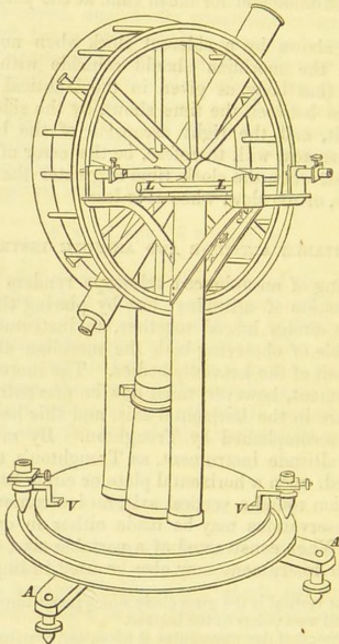
The tripod, A A, is supported by three foot-screws, by which the vertical axis is brought into adjustment, and carries the lower horizontal plate, which is graduated to show the azimuths or horizontal angles. The vertical axis is a solid
