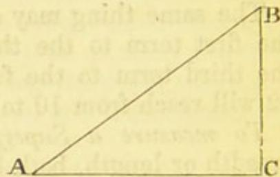
*Solution.*—Extend the compass from  $90^\circ$ , or radius, on the line of sines to the number of degrees in either of the acute angles, and that extent will reach backwards, on the line of numbers, from the hypotenuse to the side opposite this angle. *Example.*—Given the hypotenuse  $AB = 250$ , and the angle  $A = 35^\circ 30'$ .
