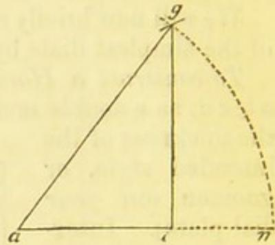
*To make an erect South Dial.*—Take the complement of the latitude of the place, which for London is  $90^\circ$  less  $51\frac{1}{2} = 38\frac{1}{2}$ , from the scale of latitudes, and proceed in all other respects for the hour lines, as above, for the horizontal dial; only reversing the hours, and limiting them to the 7; and for the gnomon making the angle of the style's height equal to the colatitude  $38\frac{1}{2}$ .
