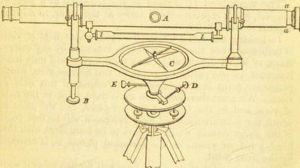
The above figure represents this instrument. A is an achromatic telescope, resting upon two supporters, which in shape resemble the letter Y, and are consequently called the
