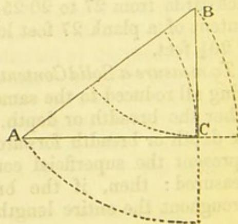
Extend from  $90^\circ$  to  $35^\circ 30'$  on the line of sines, and this extent will reach from 250 to 145 on the line of numbers . . .  $\therefore BC = 145$
