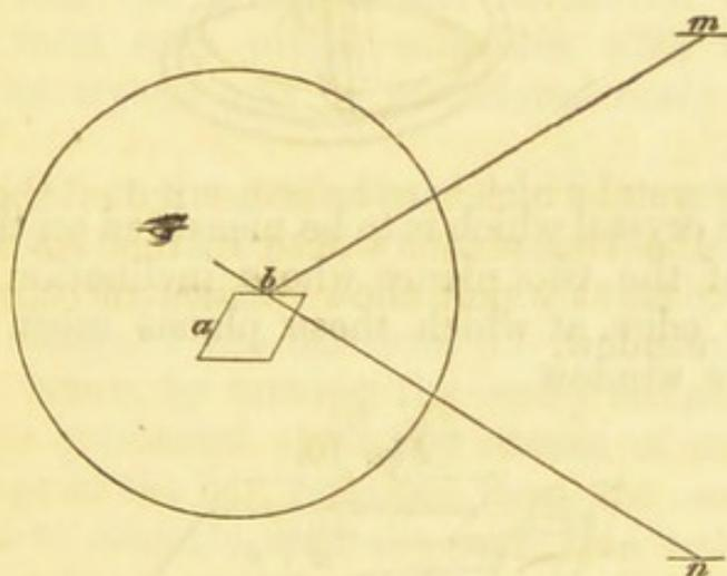
“ This purpose is effected by causing an object, as the line at *m*, fig. 8, to be reflected successively from the two planes, *a* and *b*, at the same angle. It is well known that the images of objects are reflected from bright planes at the same angle as that at which their rays fall on those planes; and that when the image of an object reflected from a horizontal plane
