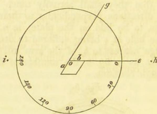
“Let  $ab$ , fig. 6, represent a crystal, of which one plane only is visible in the figure, attached to a circle, graduated on its edge, and moveable on its axis at  $o$ ; and let  $a$  and  $b$  mark the position of the two planes whose mutual inclination is required.
