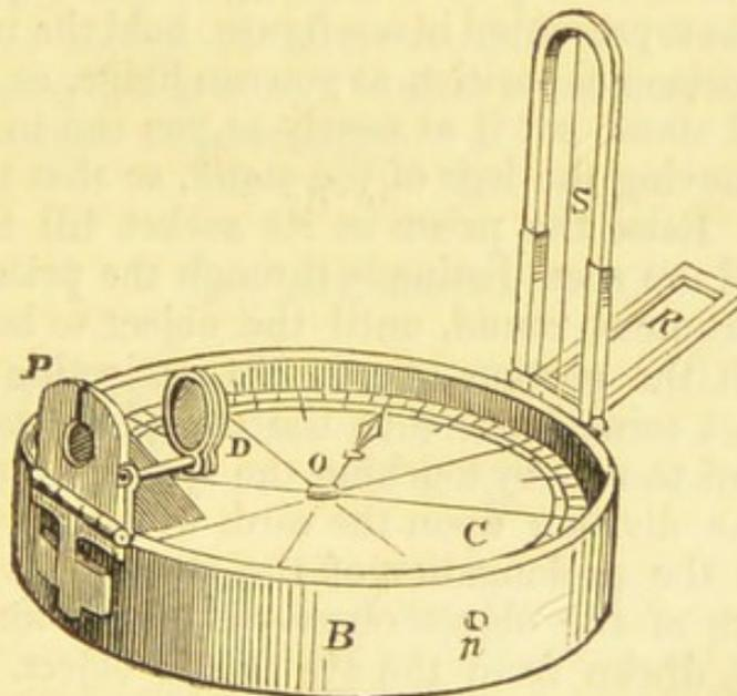
c is a compass card divided usually to every 20', or third part of a degree, and having attached to its under side a magnetic
