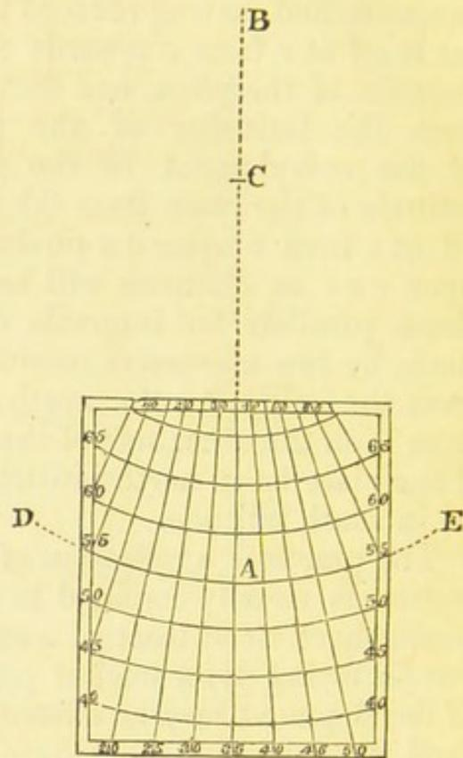
In drawing a map of small extent, it is usual to make all the meridians and parallels of latitude straight lines; and to make the extreme parallels, and the meridian passing through the center of the map, proportional to their real magnitude.
