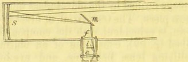
axis of the telescope, placed between the object-speculum and its focus, and an eye-piece. The pencils of light proceeding from a distant object tend to form an image after reflection at the object speculum, but are bent by the plane reflector, so that the image is formed at *i*, on the axis of the eye-piece, and in the focus of the eye-lens.
