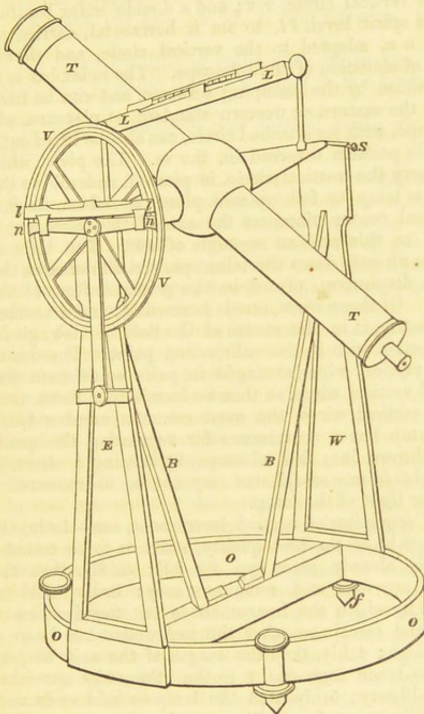
The *ys* are supported upon the standards *E* and *w*, of which *E* may be called the eastern, and *w* the western standard; and one of the *ys* is fixed in a horizontal groove, on the western standard, so that, by means of the screw *s*, one end of the axis may be pushed a little forwards or backwards, and a small motion in azimuth be thus communicated to the tele-
