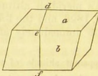
"The mutual inclination of any two planes, as of  $a$  and  $b$ , fig. 1, is indicated by the angle formed by two lines,  $ed$ ,  $ef$ , drawn upon them from any point,  $e$ , on the edge at which they meet, and perpendicular to that edge.
