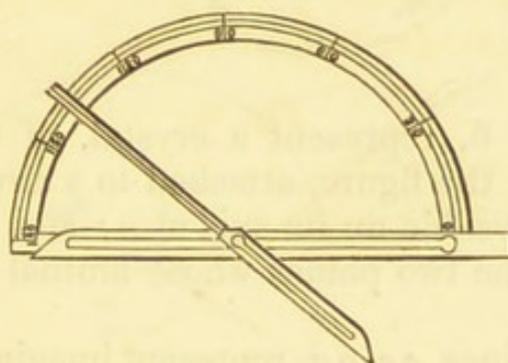
“When this instrument is applied to the planes of a crystal, the points,  $d$  and  $f$ , fig. 4, should be previously brought sufficiently near together for the edges,  $d e, e f$ , to form a more acute angle than that about to be measured. The edges being then gently pressed upon the crystal, the points,  $d$  and  $f$ , will be gradually separated, until the edges coincide so accurately with the planes that no light can be perceived between them.
