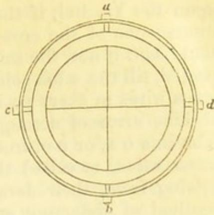
When the instrument is in adjustment, the axis of the tube of the telescope is set truly horizontal by means of the level beneath it, and the line of observation ought consequently to be parallel to this axis. Let *A* represent the proper position of the intersection of the cross wires, and *o A*, the direction of the axis of a pencil of light passing through the object-
