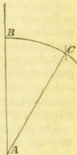
ship is to be sailed from the point A to a point on the line AC on a chart, draw meridian AB, describe arc BC with radius equal to chord of  $60^\circ$ , as before, and the extent from B to C, applied to the line of rhumbs, will give 2 pts. 3 qrs., denoting that the ship must be sailed by the compass N.N.E.  $\frac{5}{4}$  E.
