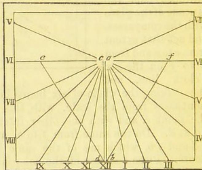
*To construct an East or West Dial.*—Draw the two meridian lines as before, and intersect it at right angles by another
