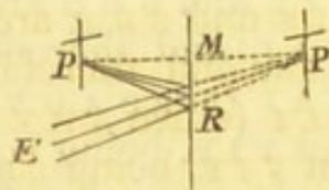
The uses of a single plane reflector in mathematical instruments are nearly the same as the uses of a prism: viz. either to alter the apparent position of an object so as to make its visual image coincide with the real image of some other object, as in the prismatic compass\*, or merely to change the direction of the pencils for the purposes of more convenient observation, as in the Newtonian telescope †, the diagonal eye-piece ‡, &c.
