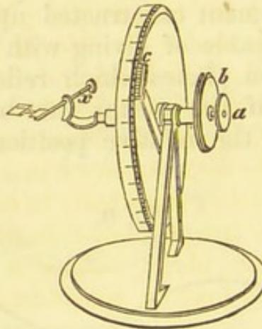
“ Place the crystal which is to be measured on the table, resting on one of the two planes whose inclination is required, and with the edge, at which those planes meet, nearest and parallel to the window.
