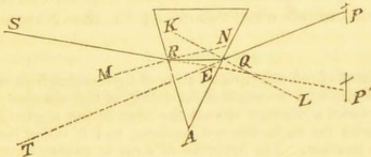
appears lower than it really is, while, if the prism were held with its edge upwards, the object would appear in a position higher than its actual position. 2ndly. The boundaries of the object are indistinctly defined and fringed with colours.
