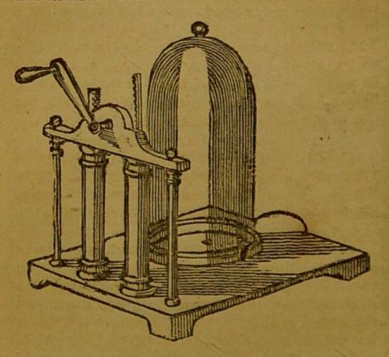
The Air Pump.—The above figure represents the cheapest form, and in action it exactly resembles the common sucking pump, with this difference, that the valves are made of moistened bladder instead of leather.
