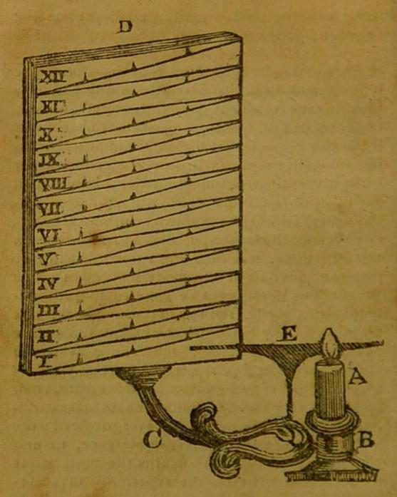
The Lamp Chronometer.—It represents a chamber-lamp, A, consisting of a cylindrical vessel made of tin, in the shape of a candle, and is to be filled with oil. This vessel should be about three inches high, and one inch diameter, placed in a stand B. The whole apparatus of lamp and stand can be purchased, ready made, at any tin shop in London. To the stand B is fixed the handle C, which supports the frame D, about twelve inches high, and four inches wide. This
