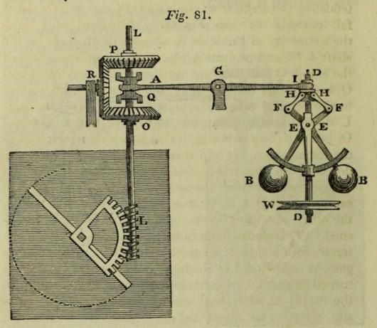
Under the circumstances here explained the shaft L M is at rest, having the bevelled wheels O P turning freely on it in opposite directions, and the machinery is supposed to be moving with the proper velocity.
