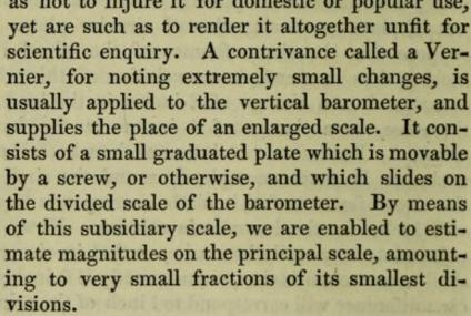
The principle of the vernier is easily explained. Let B A, fig. 16., represent the scale D of the barometer extending through three inches and divided to tenths of an inch. Let CD be 12 the sliding scale of the vernier, equal in length 8+ +3 to eleven divisions of the principal scale, and +4 divided into ten equal parts.
