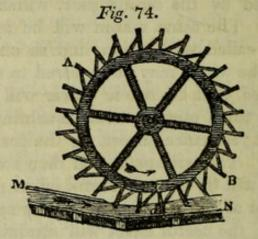
point, is immersed in a stream, called a mill-course, and the float boards are intended to receive the impulse of the water as it passes under the wheel. The wheel is thereby caused to revolve in the direction of the stream, with a force depending on the quantity and velocity of the water, and the number, form, and position of the float boards.
