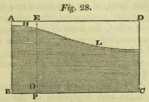
parts, a communication, O, at the bottom; and let this partition so divide the liquid, that the higher part of the surface, H, shall occupy one division, and the lower part, L, the other. We should thus have a liquid in communicating vessels standing at different levels; a result which would be inconsistent with what was formerly proved. Therefore it follows, that all parts of the surface of a liquid contained in any vessel must stand at the same level when at rest.
