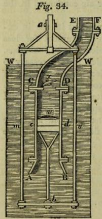
submerged in the well or reservoir from which the water is to be raised. This cylinder communicates by a valve w, with a tube or pipe CE, which is carried upwards to whatever height it is required to raise the water. A piston moves water-tight in the cylinder AD, and is worked by a rod or framework, as represented in the figure. This piston is furnished with a valve v, which opens upwards.
