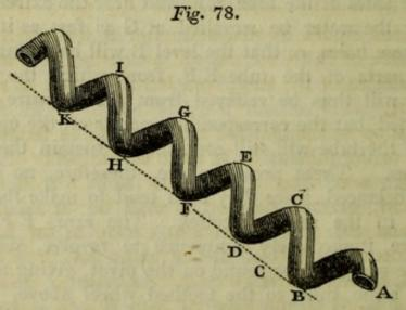
Suppose A the extremity to be open and presented upwards, and suppose the screw to be placed in an inclined
