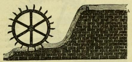
a velocity corresponding to the height of this fall rushes against the float boards, and puts the wheel in motion. The mill-course then has a further fall M V N to carry off the water, which would otherwise impede the advancing float board.
