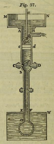
the external water in the well, because both are subject to the same atmospheric pressure; but when the syringe B C is worked it will rarefy the air in the tube S O, on the principle and in the manner explained in (148.). The pressure of the air in S O on the surface
