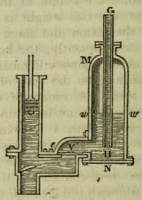
the force pipe, as already described in the suction pump, may serve the purpose, but it is generally more convenient to use an apparatus called an air vessel, which is represented in fig. 39. Immediately above the valve
