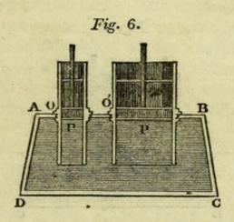
A force of a pound acting on the piston P, fig. 6., holds in equilibrium a force of ten pounds acting on the piston P'. In this case, however, it must not be supposed that the piston P supports the ten pounds which press down the piston P': the bottom of the vessel sustains by its resistance nine of the ten pounds acting on the piston P' and the remaining pound alone is resisted by the piston P.
