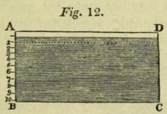
Let A B C D, fig. 12., be a vessel with a flat square bottom and perpendicular sides; and suppose it filled with water; and let the side A B be supposed to be divided into ten equal parts, marked by the numbers 1, 2, 3, 4, to 10: the pressure at the point 1 we shall suppose to be one pound. The point 2 being at twice
