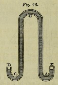
water will be driven from E with a force equivalent to the hydrostatic pressure on the surface D.
