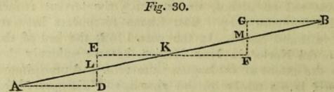
and MGB, and partly by excavations, ADL and KFM. The canal is carried successively along each of the levels BG, FE, DA. These communicate with each other by locks at ED and GF, by means of which vessels passing in either direction are raised or lowered with perfect ease and safety.
