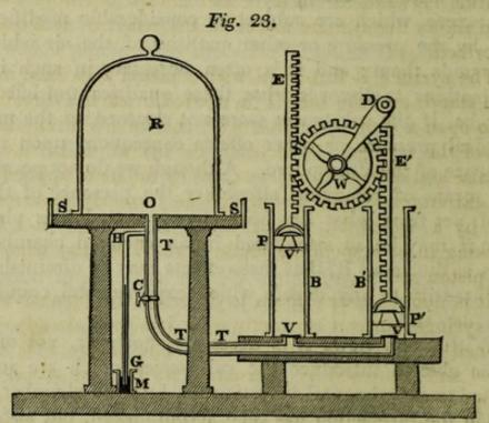
or lower part is open, and it is ground to a perfectly smooth and flat edge. A circular brass plate is constructed, also ground truly plane and perfectly smooth, and its magnitude is accommodated to the size of the largest receiver intended to be used; a section of this plate is represented at S S.
