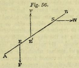
position of the vessel; let S represent the point at which the wind acts upon the sail, and let S W represent the direction of the wind: let E be the centre of gravity of the vessel and her cargo, and let E F be the direction in which her weight acts.
