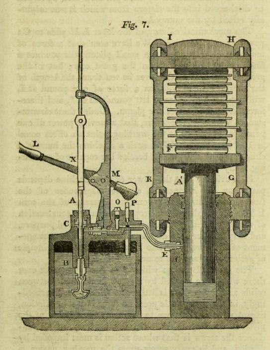
to open the screw valve-cock P. The water will be forced by the weight of the great piston A' through the tube E, and, passing through the tube of communication to which it is admitted by the open stop-cock P, it will be discharged into the cistern from which it was origin-
