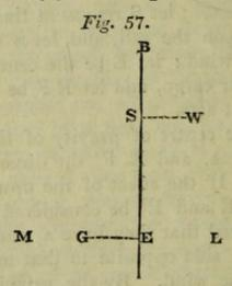
centre of gravity when over the keel, and let G represent the point to which the centre of gravity is transferred by moving the carriages to the side of the vessel; let S be the point where the wind acts upon the sail S W; the weight of the vessel acting at G, has a tendency to make it incline towards M; and the force of the wind, acting at S in the direction S W, has a tendency to make it incline towards L. These two forces counteract each other, and the vessel maintains its upright position.
