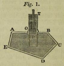
To render this property intelligible, let us suppose a close vessel of any form, such as ABCDE, fig. 1., having an aperture at O in which a tube or cylinder, OT, is inserted. Let us conceive this vessel completely filled with liquid to the level of the mouth, O, of the aperture. Let us now suppose a solid piston or plug, P, inserted in the tube, and pressed downwards until it comes into contact with the liquid. If the piston thus
