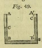
Let BB', fig. 49., be a horizontal tube connected with two upright tubes, AB and A'B', and let a stopcock be placed at B'. Let the horizontal tube BB' be filled with quicksilver, and let two liquids lighter than quicksilver, and which, bulk for bulk, have different weights,
