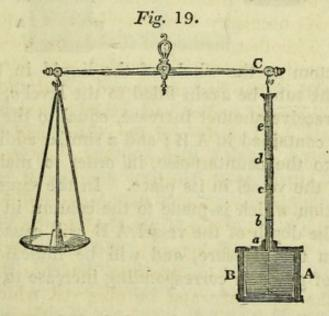
terpoised by a weight in the dish suspended from the other arm. Suppose the vessel AB now to be filled with water to the neck, a; and let the tube be divided into parts at b, c, d, e, each of which shall be equal to the depth of the vessel AB. Let a sufficient weight be put into the dish to maintain the bottom of the vessel AB in its place. This weight will be found to be equal to the weight of the water contained in the vessel AB.
