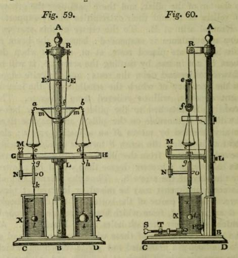
to the amount of half a grain, that being the weight which an inch of the wire loses by immersion. In like manner if d preponderate, the wire k l will be drawn up; and for every inch which is raised above the surface of the
