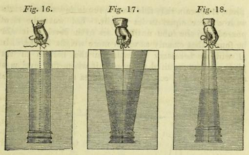
inserted in it water-tight at a, and is provided with a moveable bottom, which, however, fits it water-tight. This bottom is supported by a wire, which passing up the tube is attached to the arm of a balance, and is coun-
