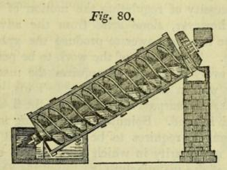
water-wheel, worked in a corresponding wheel on the other extremity of the shaft. The screw was thus kept in constant revolution by the fall of water which supplied the reservoir, from whence the same water was to be raised by the screw itself.
