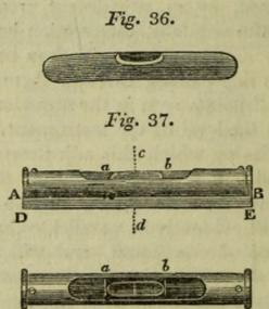
The method of mounting the level for the purpose of fixing a plane in a horizontal position, is commonly to fix the tube in a block of wood, or in a case of brass, A B, fig. 37. The block is fixed in such a position, that when the lower surface, D E, is horizontal, the bubble will stand in the centre between two lines, a and b, cut upon the tube. The instrument may be adjusted by the following method: — Let a plane surface be con-
