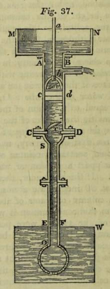
raised in the tube S O, will be less than even 30 feet in height. It is obvious, however, that within this limit the length of the tube S O must be determined by the degree of excellence attained in the construction of the syringe C B.
