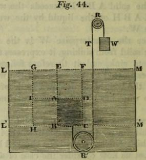
Finally, let us consider the case in which the solid immersed has a tendency to rise to the surface; suppose a fine thread attached to the bottom of the solid to be carried under a grooved wheel R', fig. 44., and, being
