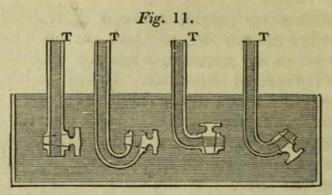
water. The water will then press against each of the cocks with a certain force, the amount of which it is required to ascertain. We shall suppose the bores of the tubes to be equal, although that circumstance, as will hereafter appear, cannot affect the result of the experiment. Let us suppose the diameter of the bores of each of the tubes to be half an inch.
