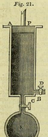
piston be pressed to the bottom of the barrel as before, the air contained in the cylinder will again be expelled through the stopcock D. By continuing this process, alternately opening and closing the two stopcocks, and elevating and depressing the piston, a quantity of air will rush from the vessel R on each ascent of the piston, and the same quantity will be expelled through the tube D on each descent of the piston.
