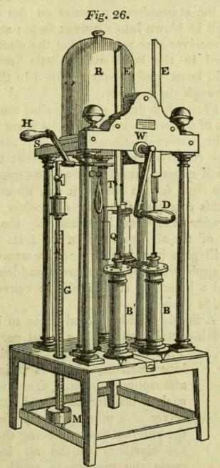
of the external atmosphere on the bladder will immediately cause its upper surface to be concave, and when the air is sufficiently rarefied within the receiver, the pressure on the bladder will burst it, producing a loud noise like the discharge of a pistol.
