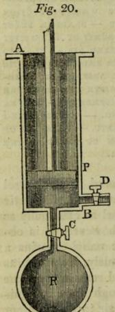
A B, fig. 20., a cylinder, or barrel, furnished with a stopcock C, inserted in a small aperture in the bottom. Let the end of this tube be screwed upon the vessel R, in which the rarefaction is to be made.
