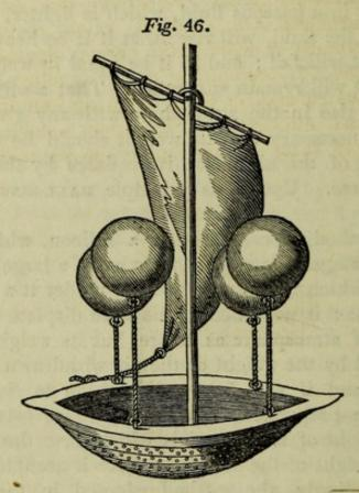
it be made of so great a thickness that its weight will very much exceed the weight of the air which it displaces.
