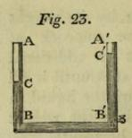
will therefore fall, and the level C will rise. When they attain the same height, their weights will mutually balance each other, as in fig. 22.; and if these were the only forces in action, all motion would then cease. But in the descent of the column B'C' the whole mass of liquid
