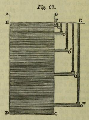
and consequently the liquid must rise to the same height before it loses the velocity with which it was discharged. Hence the jets severally issuing from the orifices will rise to the height F G.
