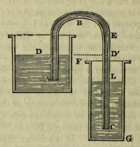
the water rises in the vessel F G, the actual leg of the siphon is shortened. When the surface L has risen towards the level of the surface D, then the legs of the siphon become equal, and, by what has been already stated, its action must cease.
