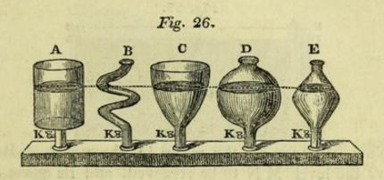
they attain the same level, and then all motion will cease. If the stopcocks be again closed, and water poured into the vessels, so as to give the liquids different levels, the experiment may be repeated by opening the stopcocks. It will always be found, that, when the stopcocks are opened, the liquid will settle itself to the same level in all the vessels.
