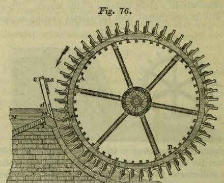
in contact with it. The spaces enclosed by the float boards and the mill-course thus serve the same purpose as buckets in the overshot wheel, and the water enclosed in them turns the wheel by its weight.
