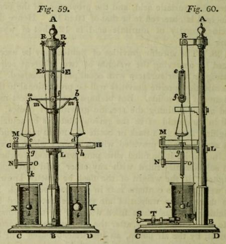
extreme accuracy is sought, the measurement of specific gravities is effected by a very sensible balance furnished with certain additions, and mounted in a manner from
