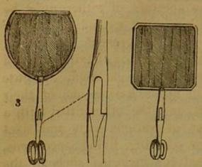
5 or 6 inches in diameter will be a very good size; the joint of the handle should be placed nearer the rings for the thumb and finger than to the leaves, or the instrument will not open well. Green gauze or transparent muslin is fastened tight round
