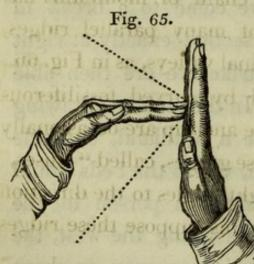
may measure the angle within a few degrees by standing exactly opposite to a cliff where the true dip is exhibited, holding the hands immediately before the eyes, and placing the fingers of one in a perpendicular, and
