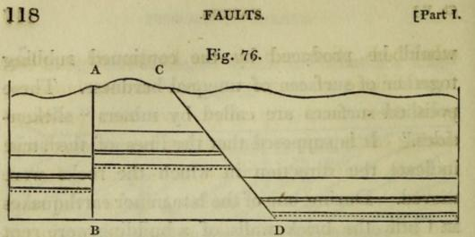
Faults. A B perpendicular, C D oblique to the horizon.
