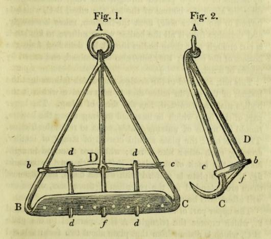
To have a clear idea of the dredge, and the parts which compose it, we must imagine a circular bar of iron, forged in the shape of an almost equilateral triangle, A, B, C, of the above figure, whose two extremities are joined at A. To form the summit or point of the triangle, each of the sides should be above five feet. The two branches, A B, and A C, are rounded and bent, as they approach the base of the triangle. The base, B C, is forged into a plate, six inches in breadth with a sharp
