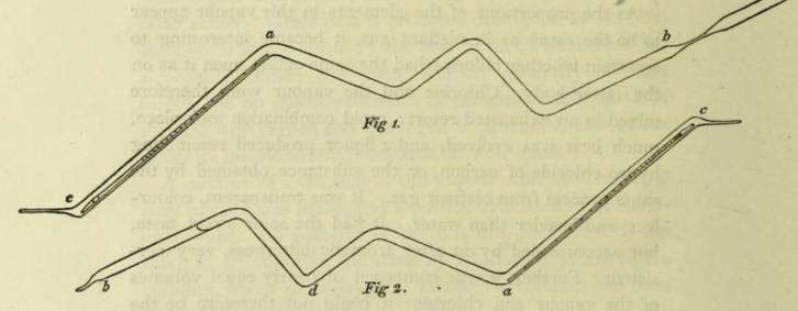
gauge at a. c. and the extremities being open. It was then cooled to  $o^{\circ}$  from a to b, and in that state made the receiver into which the first product from a portion of the original fluid was distilled. The part at b was then closed by a spirit lamp; and having raised enough vapour to make it issue at
