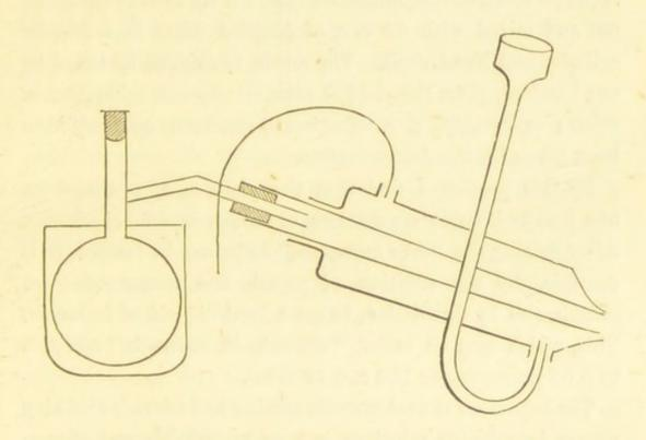
should be lowered. This is done by getting the flask out of the hot oil or spermaceti, and either the oil-bath may be lowered down away from the flask, or else the flask, which is to be maintained in firm connection with the Liebig's condenser, may be raised out of the oil.
