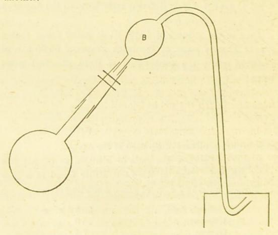
The gases in water are estimated by taking a known volume of water, boiling out the gases, and collecting them
