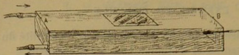
Fig. 88. — Platine chauffante de Pfeiffer.
