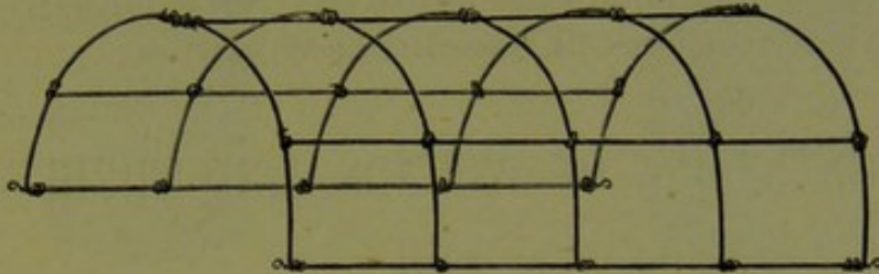
Cradle of iron-wire, easily made of telegraph wire.
