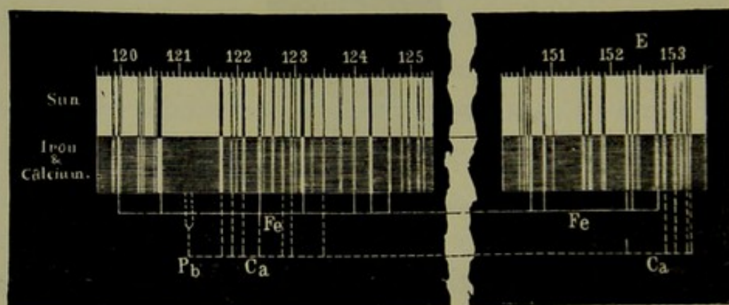
Coincidence of the Fraunhofer Lines with the Lines of Iron and Calcium.
