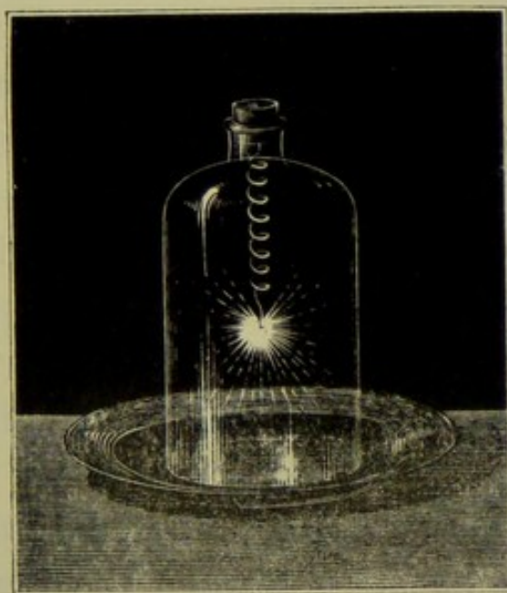
Combustion of a Steel Watch-spring in Oxygen.
