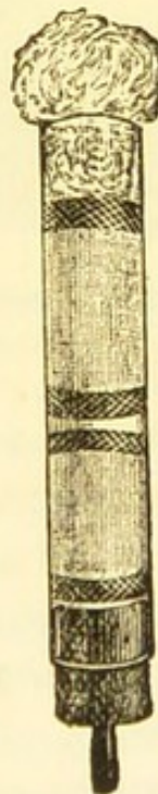
FIG. 113.—Filtering tube to keep back the bacteria.
