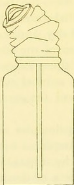
FIG. 31.—The flexible bellows-pump employed by Angus Smith to draw out air from the air-jar.
