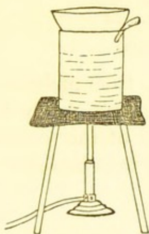
FIG. 19.—A water-bath improvised from an ordinary beaker.
