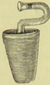
FIG. 9.—Poltzer's ear manometer.
