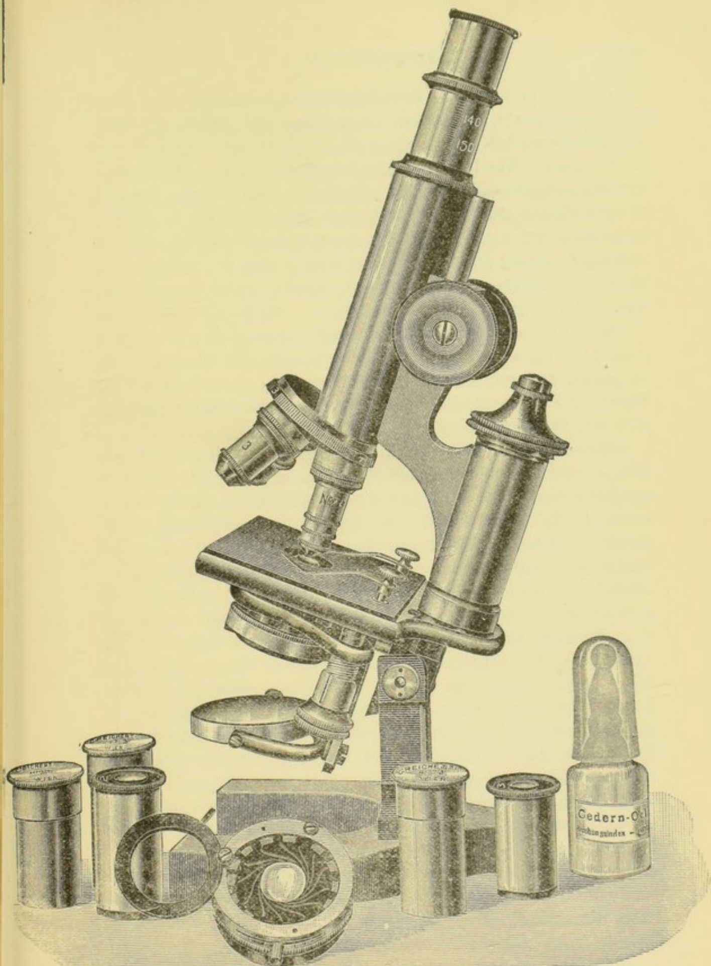
Fig. D.—Reichert's stand No. IIIb, showing objectives, eye-pieces, iris-diaphragm, Abbe condenser, and round, dustless nose-piece.
