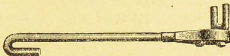
FIG 21. Thomas' Wrench for bending the splint, modified from Moore's triple-action ratchet-drill, and made by the Lowell Wrench Co., of Worcester, Mass. (Ridlon.)
