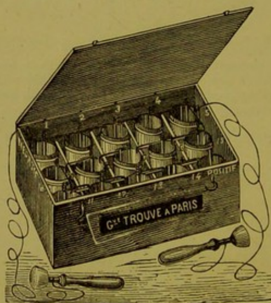
A battery of 15 Callaud-Trouvé elements in a box. The rheophores are connected by means of clips to the wires binding the elements together.
