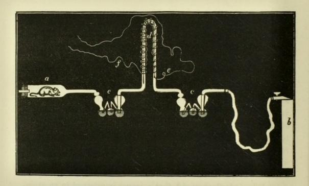
Description of Figure.—a, glass chamber for reception of the animal; b, gasometer; the current of air or gas passed from right to left of diagram; c (to the right), bulb-tube containing sulphuric acid; c (to the left), bulb-tube containing caustic potash or water; d, U tube; e, wire from — pole of induction coil continuous with platinum wire within the U tube; f, wire from + pole of induction coil continuous with copper wire coiled round U tube.
