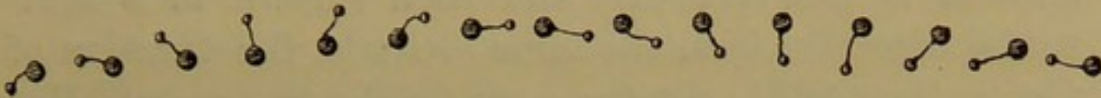
FIG. 57.—Movement of a system of two balls bound together by a string.
