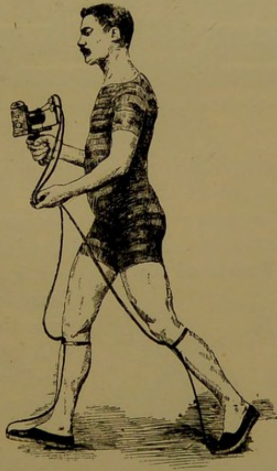
FIG. 4.—Pedestrian furnished with special shoes and carrying a chronographic apparatus.
