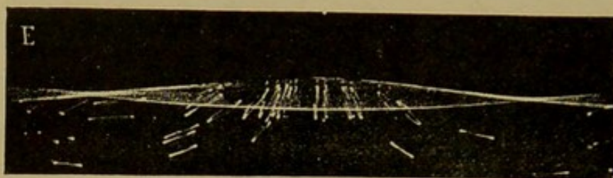
FIG. 62.—Molecular movements within a simple chopping wave.
