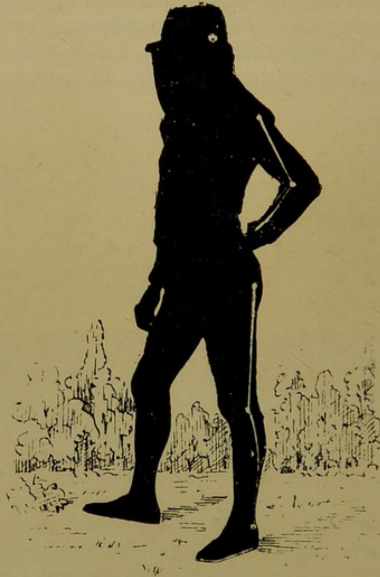
FIG. 41.—Man dressed in black, with white lines and points for the chronophotographic study of the movement of the important parts of the body.
