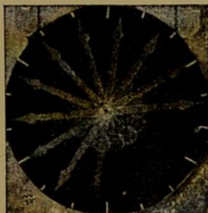
FIG. 12.—Successive positions of the needle on the chronometric dial, measuring the intervals of time separating the successive exposures.
