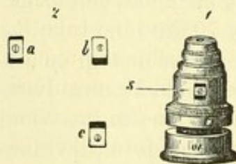
Fig. 19. Achromatic objective with correcting apparatus.
