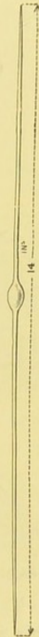
FIG. 5—A CAPILLARY PIPEPTE, DRAWN OUT INTO FINE POINTS; LENGTH ABOUT 12 TO 14 INCHES.
