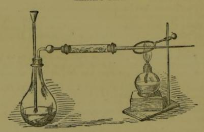
Marsh's Test depends upon the formation of arseniuretted hydrogen. I must explain here that arsenic, arsenious acid As<sub>2</sub> O<sub>3</sub>, is not, as I have said, an acid at all; it is in fact tasteless, and is only called an acid in the inaccurate jargon of science becauseit possesses a property common to acids, it combines with alkalies. Arsenic is, in fact, an anhydride, and is sometimes, and more accurately, called "anhydride," which means that there is no hydrogen in it.
