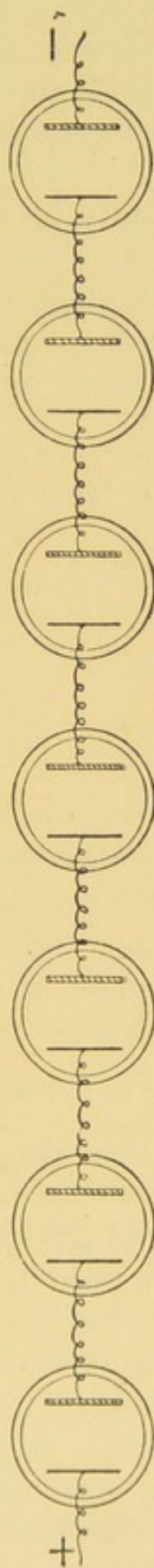
FIG. 27.—PLAN OF SEVEN CELLS IN SERIES.
