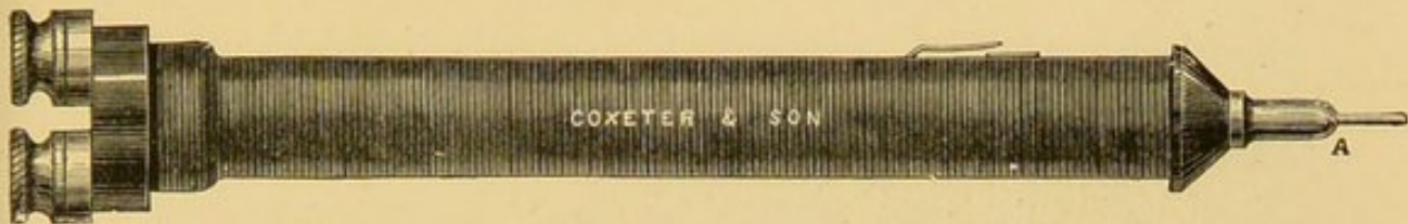
FIG. 127.—ELECTRO-MAGNET FOR OPHTHALMIC PRACTICE.
