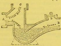
Fig. 20.—Disconnecting and Ventilating Drain Trap No. 2, Buchan's Patent.
