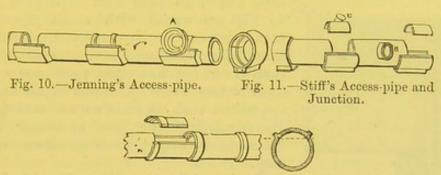
Fig. 12.—Doulton and Watt's Access-p'pe.
