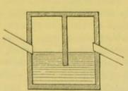
Fig. 16.—Common Mason's or Dip-Trap. Bad form of Trap.
