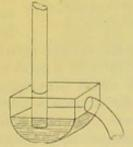
Fig. 17.—D Trap. Bad form of Trap.
