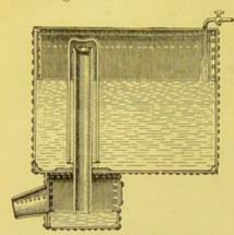
Fig. 13.—Field's Flush Tank.
