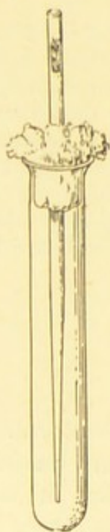
FIG. 44.—Test-tube and pipette arranged for obtaining fluids containing bacteria.
