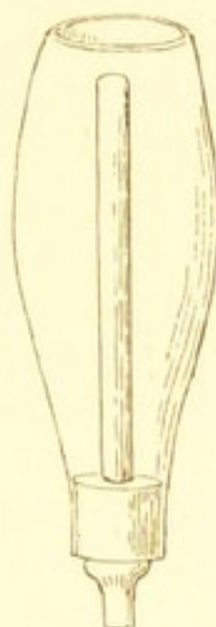
FIG. 33. — Bougie inserted through rubber stopper for same purpose as in Fig. 32.
