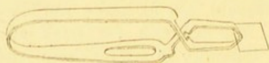
FIG. 40.—Cornet's forceps for holding cover-glasses.
