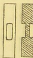
Fig. 108.—Method of cutting strips of plaster.
