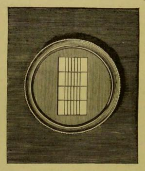
Fig. 26.-Micrometer Screen for Ophthalmoscopic Measurements.
