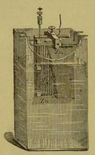
FIG. 59,—SMEE BATTERY WITH-OUT DEPOLARIZER.
