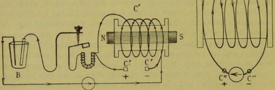
FIG. 3.-FARADIC APPARATUS, SHOWING CURRENT OF MAKE AND MAGNETIZATION.
