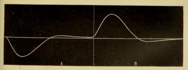
FIG. 4.—Curves Obtained by Making and Breaking the Current from an Ordinary Induction Coil without a Rheotome. A, make; B, break.
