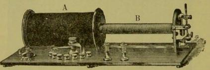
FIG. 78.—THE ROCKWELL COIL FOR CURRENTS OF QUANTITY AND TENSION.
