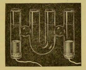
FIG. 1.-APPARATUS FOR TESTING THE BACTERICIDAL PROPERTIES OF ELECTRICITY.
