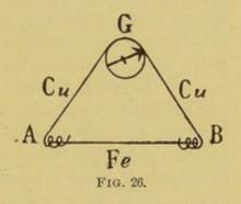
current. This can really be done, as was discovered by Peltier. His discovery was this: Pass a current through a junction of two different metals; then heat will be disengaged if the current be in opposition to the direction in which a current would be produced by heating the junction, and heat will be absorbed if the current be in the direction of the current that would be produced by heating the junction.
