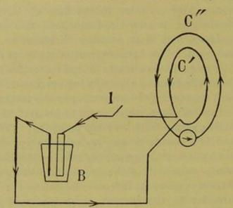
FIG. 1.—SIMPLE PRIMARY (C') AND SECONDARY (C'') CIRCUIT AT BREAK OR OPENING OF CURRENT.
