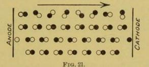
• an atom of hydrogen; O an atom of chlorine; -> direction of current.
