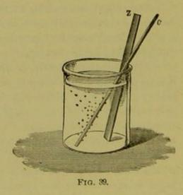
to the electrodes, and which permit the transference to a distance of the effects produced by the battery, are called *rheophores*. The *rheophores* are generally short, and often end in a longer wire, to which the name of *conductor* is given.
