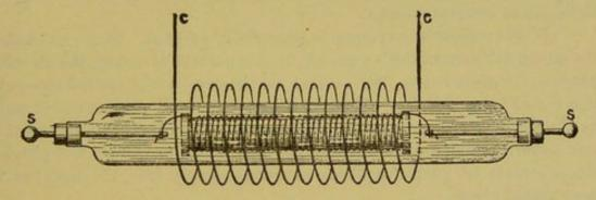
FIG. 7 .- SOLENOID AND COIL FOR USE IN CONNECTION WITH CONDENSERS.
