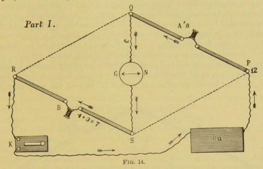
current, 3, overcomes the lesser,  $1\frac{1}{2}$ . In Part I, 4 + 3 = 7 go by *B*, and in Part II 5 go by *B'*; and if the two are added together they again make the 12 parts, which, as before, travel through the key and connecting wire to the other pole of the battery, *Ba*.
