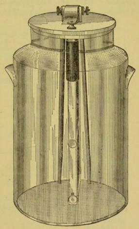
FIG. 49.-EDISON-LALANDE COPPER-OXIDE BATTERY.
