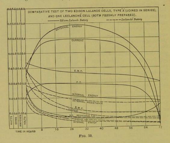
In this test the batteries were so arranged as to be alternately thrown into circuit with a resistance coil. The periods of rest and work were of five minutes' duration. When the Leclanché was resting the Edison-Lalande was working, and vice versâ.
