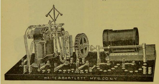
FIG. 12.<sup>1</sup>-New Engelmann Battery with Variable and Controllable Interrupter and Alternator.
