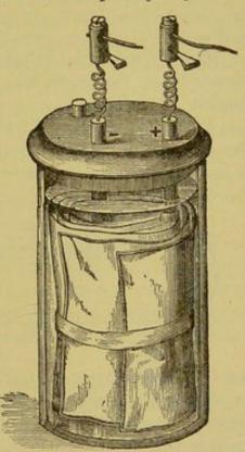
FIG. 63.—FAURE'S MODIFICATION OF THE PLANTE CELL.
