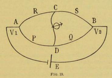
along A C B, and also along A D B. Now by Ohm's law, since the current in all parts of A C B is the same, the fall of potential in any part of A C B is proportional to the resistance of that part. Hence, if we take two points, C and D, at the same potential, then C must divide the resistance of A C B in the same proportion as D divides that of A D B. Calling the resistances of the parts P Q and R S, we have
