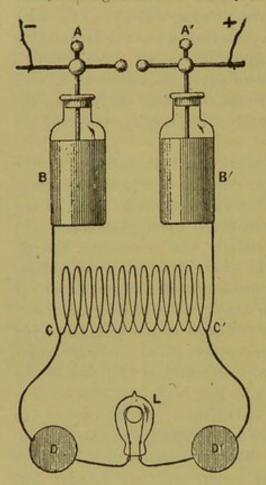
FIG. 6.—ARRANGEMENT OF LEYDEN JARS FOR PRODUCING ALTERNA-TING CURRENTS OF GREAT FRE-QUENCY. (D'Arsonval-Hertz.)
