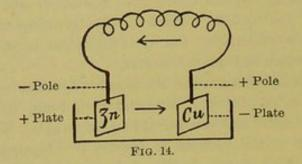
rules given in § 36, that the positive current goes from the copper plate along the wire to the zinc plate, and thence from the zinc plate in the liquid to the copper plate. (As a memoria technica, the rule zinc in liquid to copper may be shortened to z-in-c,—spelling the word zinc.)
