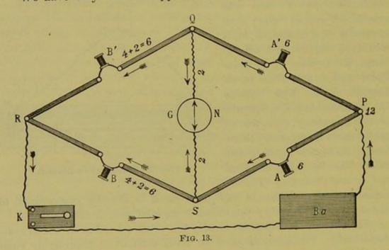
R, and 4 + 2 = 6 by S to R; the two added together make 12, the original quantity started with, which proceeds through the key and connecting wire to the other pole of the battery, Ba.
