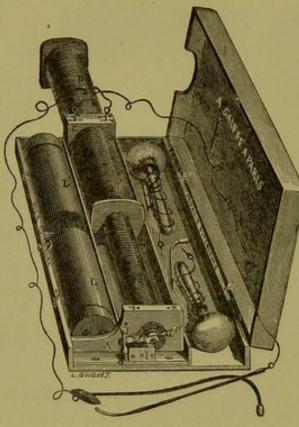
FIG. 2.-PORTABLE FARADIC BATTERY.
