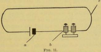
a, battery ; b, electro-magnet; c, connecting wire.
