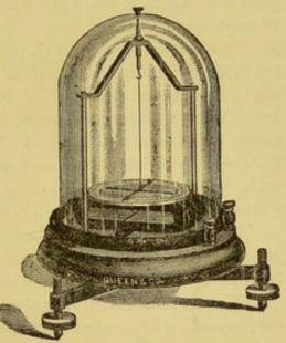
FIG. 23.-ASTATIC GALVANOMETER.
