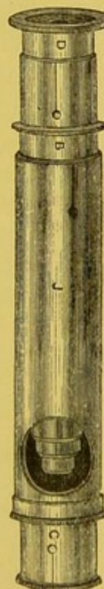
Waistcoat pocket microscope, only 4 inches long. Made by Mr. Highley. p. 16.
