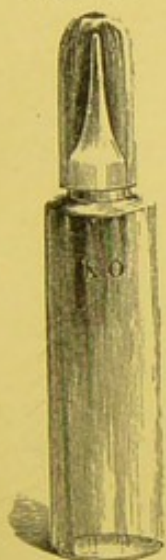
Test bottle, with capillary orifice. p. 209.
