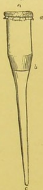
Pipette serving as the stopper to the bottle. a, vulcanised India rubber, by pressing which fluid may be expressed from the tube. b, ground to fit the neck of the bottle. c, the orifice. p. 210
