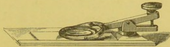
Compressorium for pressing or tearing up tissues under the microscope. p. 81.
