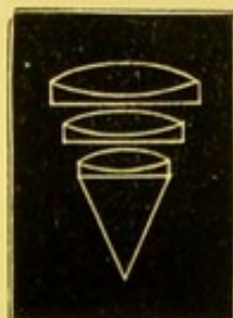
Compound glasses of an achromatic object glass. p. 6.
