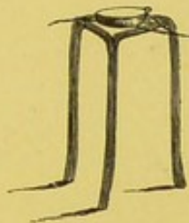
Tripod wire stand for supporting platinum. p. 43.
