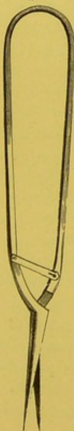
Spring scissors, for making minute dis- sections. p. 45.
