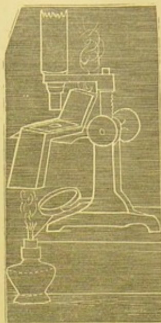
Apparatus for keeping objects warm while being examined in the microscope. p. 157.
