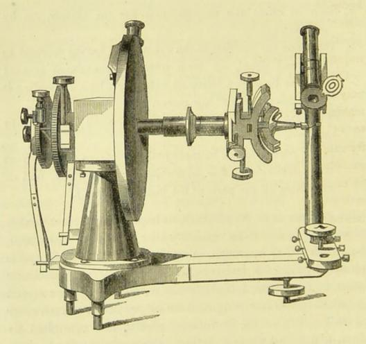
attendant apparatus of adjustment, which slides along and can be clamped to an accurately turned cylinder of steel, forming the prolongation of the axle of the goniometer. Adjustments for regulating the parallelism of the plane containing the axis of the telescope and the signal, with the plane of the goniometer's disc, and for correcting errors in all other parts of the instrument, render it, without doubt, more or less complex in use ; but, when
