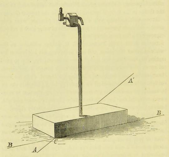
line A is ruled on the paper along the straight edge of the board. Keeping the crystal as nearly as may be over the same spot, the signals are brought into coincidence for the second face, and a line B ruled as before, intersecting with A in a point c. The angle A C B, in which the two lines, corresponding to the two positions of the instrument, intersect, is that between normals to the faces, and may be determined by the aid of a pair of compasses.
