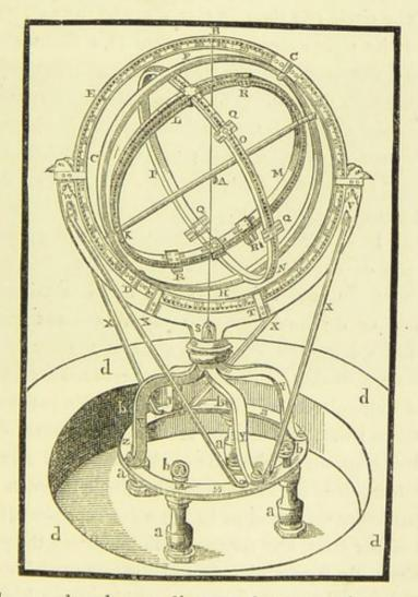
I K, which are placed at a distance from C and D equal to the obliquity of the ecliptic; so that I and K represent the poles of the ecliptic, and the circle O P the ecliptic itself. There is another circle, R M, turning on the pivots I and K, representing a meridian of longitude along which latitude is measured.
