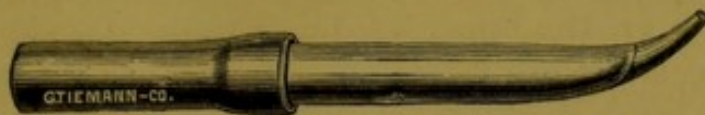
FIG. 21. Dropping tube. Pressure on the rubber expels the air from the tube. Releasing the pressure, while the tube is dipped into the solution, to be used, allows the fluid to mount in the tube. When the tube is thus charged, slight pressure upon the rubber will expell the fluid in the shape of drops, and in a quantity which can be easily regulated.
