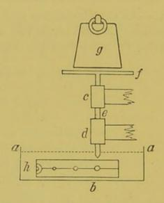
Fig. 5.—Plan of Instrument. a b a, Water cistern; dotted line, upper surface of water. c d, The fixed sheath in which moves e, the stem of f, the tray which receives g, the weight superimposed on h, the instrument perforated with three different-sized holes to receive the tangle-tents of corresponding sizes. The joint upon which the two limbs move is at h; and the holes for the tents are bisected by the line of junction of the limbs.
