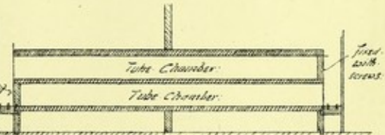
Section thro. Tube Chambers for extra long tubes.
