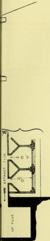
FIG. 63. PART PLAN OF CLOSETS.
