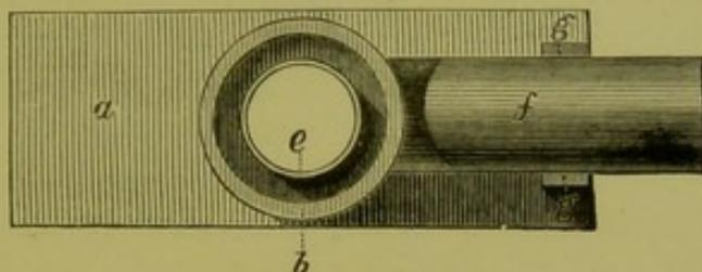
Fig. 4.—A view of the upper surface of the disc of thin brass *j*. The square of thin glass *c* is also shown in position.
