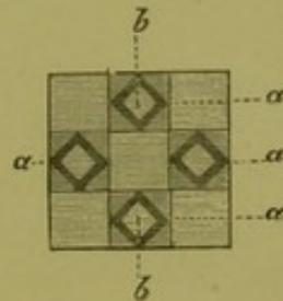
Fig. 6.—*a*, roof or cover to the stage *d*; *b*, pillar which supports the roof *a*; *c*, glass slips seven eighths of an inch square; *e*, socket which fits on to the upper part of a pillar of wood four feet six inches long, and which has its lower extremity fixed into a block of wood which rests on the ground.
