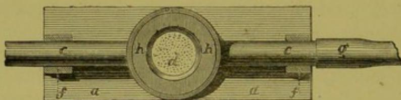
Fig. 2.—A view of the upper surface of Fig. 1. *a, a*, glass plate (an ordinary microscopic slide will answer the purpose); *c, c*, glass or brass tubes cemented to the steps *f, f*, and to the cell *b, b*, which is here concealed by the cap *h, h*; *g*, caoutchouc tube attached to the mouth-piece *e* (shown in Fig. 1), and to the tube *c*; *h, h*, brass cap which holds the disc of glass *d* in position, and covers the cell *b, b* (shown in Fig. 1).
