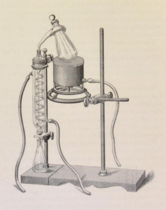
Safety funnel, as in figure, for introducing liquids into the alembic. The bowl should hold about 50 c.c., and the inside diameter of the tube be about one-quarter inch. The lower end of the tube is protected by an outside tube, which renders it much easier to withdraw the funnel without soiling the neck of the alembic.
