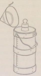
Great care must be taken in collecting water samples, in order to secure a fair representation of the supply and to avoid introduction of foreign matters. The five pint green glass stoppered bottles used for holding acids are suitable for containing the samples. The contents of two such bottles will suffice for most sanitary or technical examinations, and frequently only one will be required. The annexed cut shows a permanently
