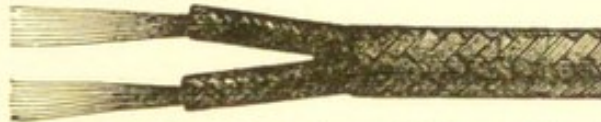
Fig. 13—Double Conduction Coil made of 16 strands of No. 33 copper wire, with silk braid cover.
