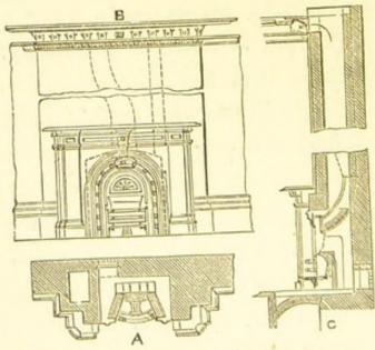
Captain Galton's Vertical Stove. A, plan; B, elevation; c, section. (I.) In Captain Galton's stove \* the air is warmed in chambers behind the grate. The point of dis-\* This stove seems to be in use in several cottage hospitals.
