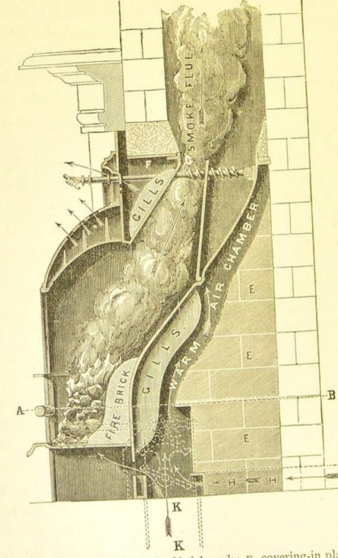
E, E, E, air chamber formed of brickwork; F, covering-in plate, resting on bar G to render the joint air-tight.
