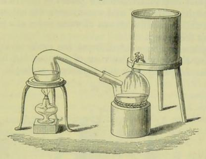
ency. The following illustration (fig. 45) represents a form of still, of common use in our laboratories, for distilling water. The kettle A, which contains the water, is covered by the
