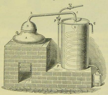
movable dome B, from which the pipe b c conducts the vapour into the receiver R, which is surrounded with cold water.
