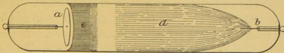
FIG. 1.—Electric discharge at a moderately low pressure. The negative electrode a is a disc, and is separated by a small dark interval from the blue negative glow c . The glow along the rest of the tube to the anode b is, in air, a diffuse band of reddish light, d .
